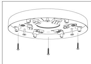
Fixate the mounting plate to the ceiling with screws.
