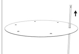
Lead the cables through the cover plate.
