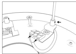
Lead the cables through the cable relief and fixate the cable by turning the screw clockwise.
