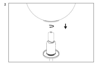
Take the glass globe and carefully place it over the diffuser. Fixate it by turning the glass globe clockwise.
